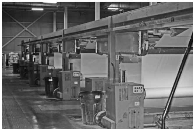
FIG. 6—A production run of 20 lb. multipurpose paper. The webs of paper from the six feeder rolls come together as layers at the entrance to a cutting unit.
