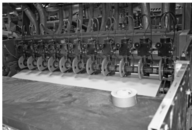
FIG. 8—Ten ribbons of 8.5" paper are cut simultaneously, just prior to being cut into 11" lengths. The rolls are 86" in width, allowing a 0.5" trim on both ends.
