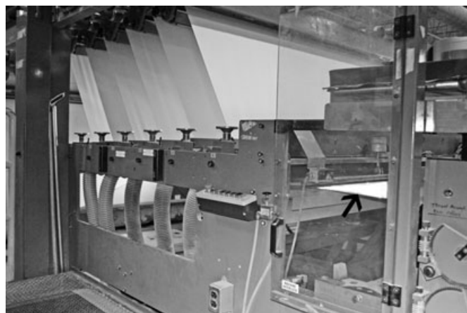
FIG. 7—Six sheets are layered together, shown by the arrow, just prior to being cut into ten, 8.5" wide ribbons. The ribbons of paper are then cut into 11 inch lengths, or other lengths according to customer specifications.
