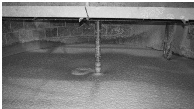
FIG. 5—The vat holds a combination of wood fibers from various tree types and several additives. The pulp is constantly stirred in preparation to be pumped to the “headbox” of a twin-wire or Fourdrinier machine.
